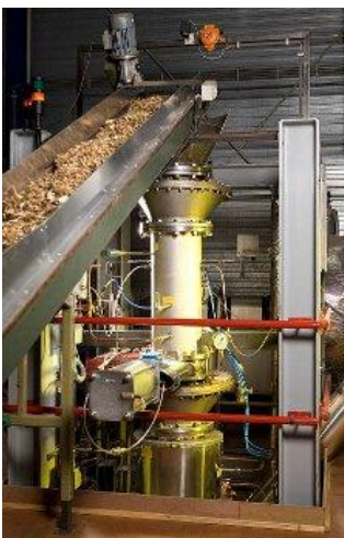
TNO's Torrefaction Pilot-scale test rig
